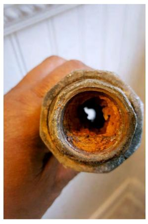
State Rep. LaTonya Johnson, D-Milwaukee, holds corroded galvanized plumbing that was removed from her Milwaukee house. Galvanized pipes, likely to be in older homes, can accumulate lead from service lines, such as the one supplying Johnson's home. Photo courtesy of the Wisconsin Center for Investigative Journalism
